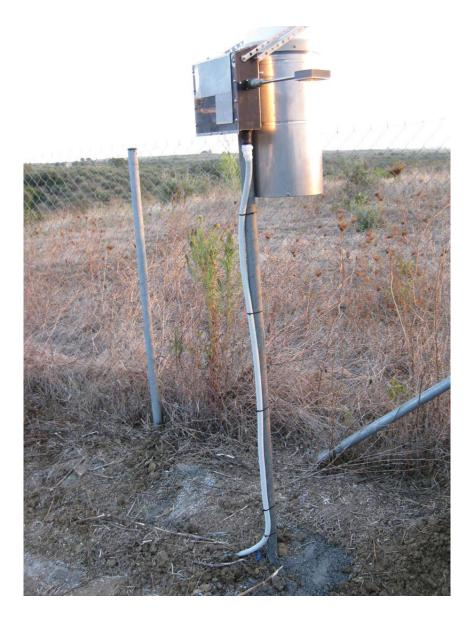
Picture 1: Rain sampler installed at Mouzaki meteorological station
