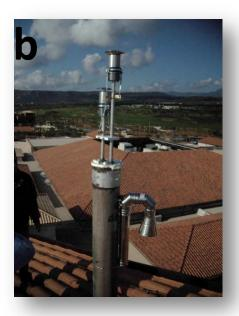
Figure 3: The atmospheric research station at the Library tower. a) The laboratory room b) Sampling heads
