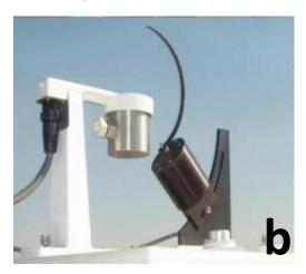
Figure 1: a)UV instrument for measurements of the Erythemal and the UVA irradiance levels, b) MFR Radiometer for measurements of diffuse and total visible solar irradiance and aerosol Optical Depth retrieval
