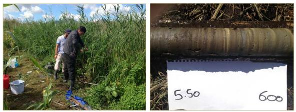
Figure 3: Coring with Russian corer in Ag. Floros.
