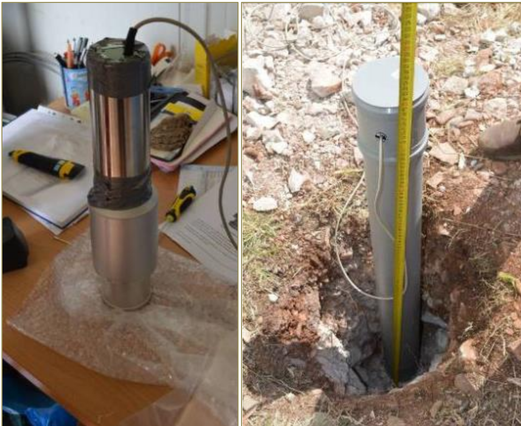
Figure 3: Detection system for the measurement and monitoring of the radon level in the soil, installed at NEO
