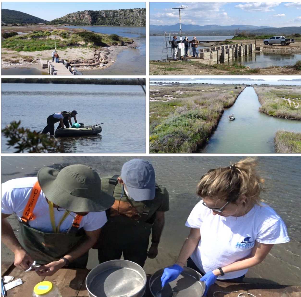
Figure 4: Top pictures: Installation of a new meteorological station with the support of the technical staff of Scient-Act. Middle pictures: Installation of new multi-parameter instrument at the wetlands of Gialova, with the support of colleagues from the Hellenic Centre of Marine Research. Bottom picture: Sampling of material for benthic analysis.
