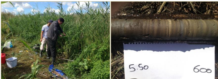
Figure 13: Coring with Russian corer in Ag. Floros.
