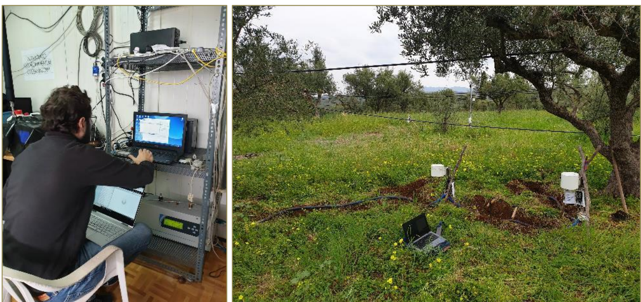
Figure 5: Left picture: Iasonas Stauroulas installing the new Nephelometer and NEO atmospheric station. Right picture: Uninstalling the soil moisture sensors at the olive orchard.
