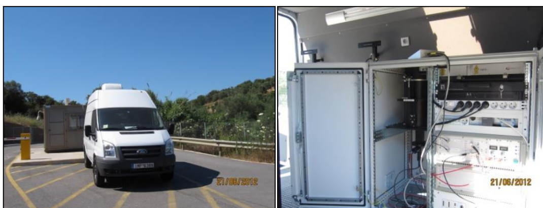
Figure 2. The LIDAR system on board of the new van type mobile lab of the AA/NEO.
